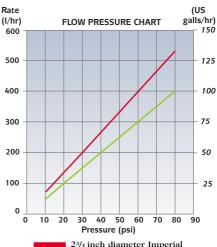
2<sup>3</sup>/<sub>4</sub> inch diameter Imperial 2 inch diameter Slimline
